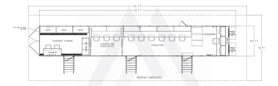
10 Working Positions 72' x 19' Recommended Working Area Single Phase, 208V, 150 Amps Cable compliment customized based on show requirements. Contact us for more information.
