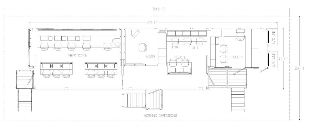
10 Working Positions 60' x 23' Recommended Working Area Single Phase, 208V, 150 Amps Cable compliment customized based on show requirements. Contact us for more information.
